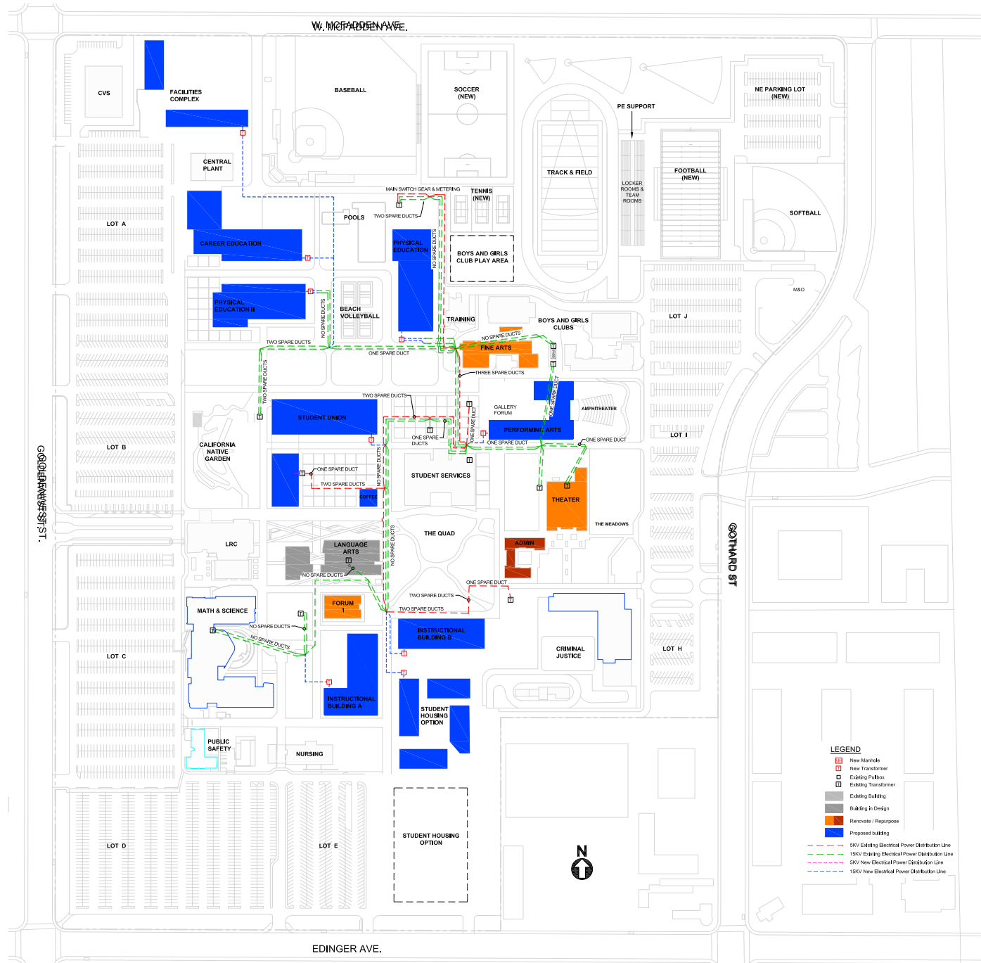
FIGURE 2 : PROPOSED 12KV AND 4.16KV POWER DISTRIBUTION SYSTEM
