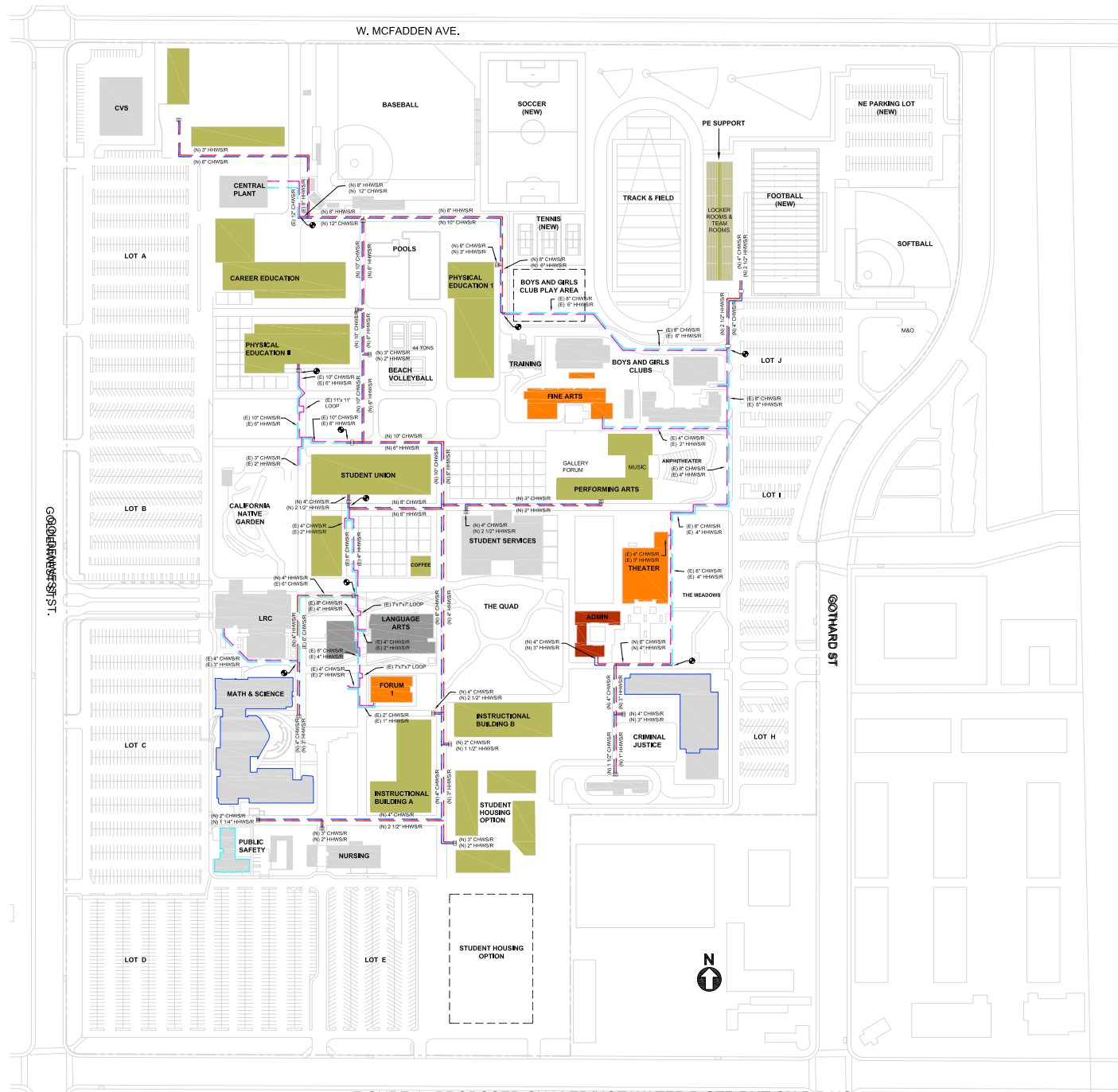
FIGURE 4 : PROPOSED CHILLED/HOT WATER DISTRIBUTION PIPING
