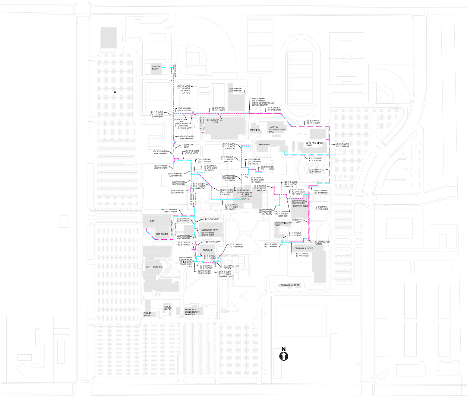
FIGURE 3 : EXISTING CHILLED/HOT WATER DISTRIBUTION PIPING (PROPOSED DEMOLITION PLAN)
